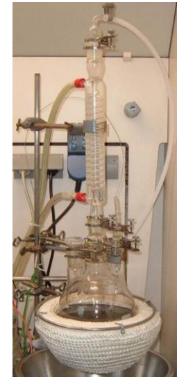
Long-term corrosion test (5000 h)
